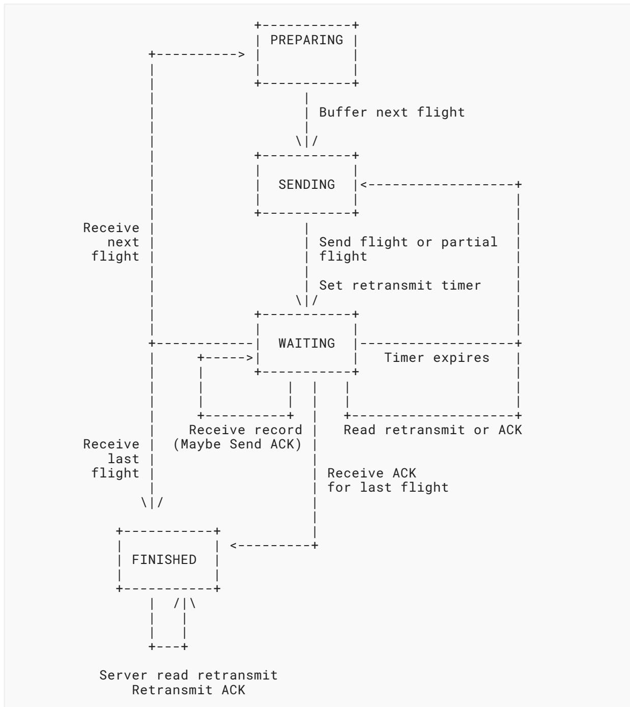
Figure 11: DTLS Timeout and Retransmission State Machine
