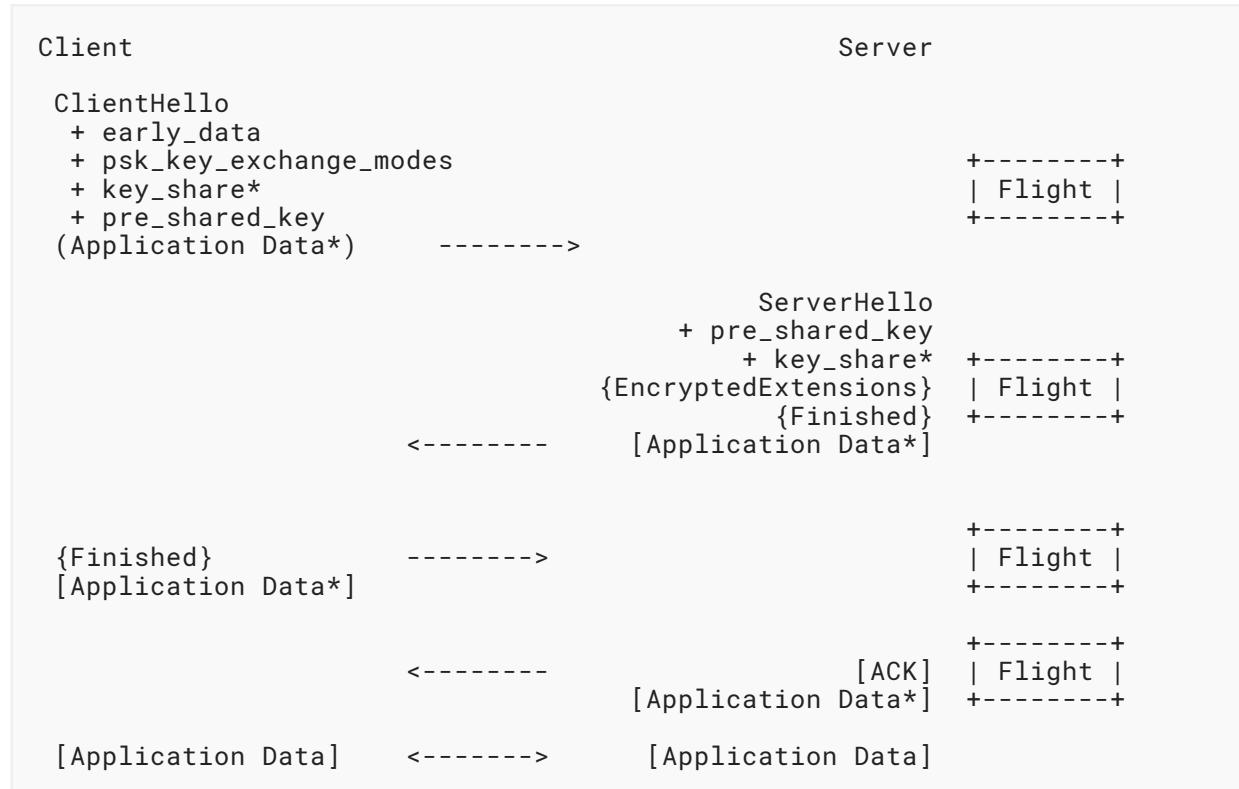
Figure 9: Message Flights for the Zero-RTT Handshake
