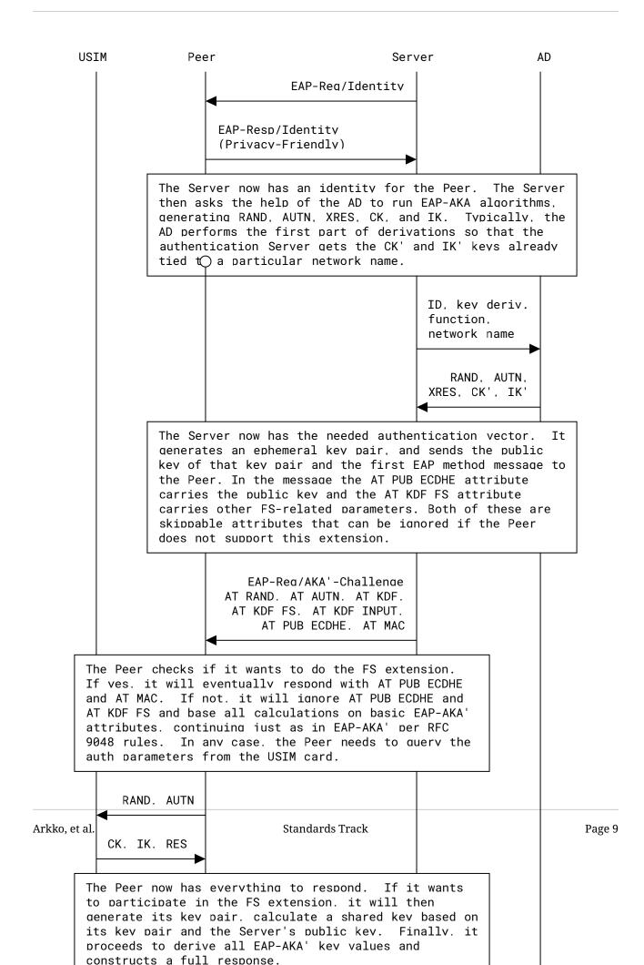
Figure 2: EAP-AKA' FS Authentication Process
