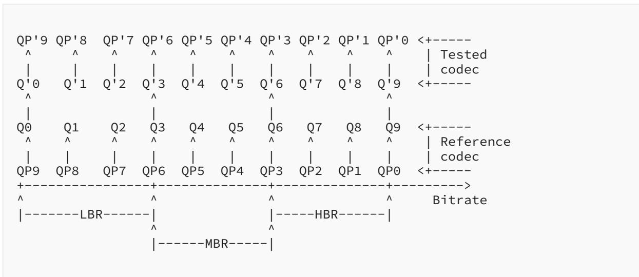
Figure 1: Quality/QP alignment for compression performance evaluation
