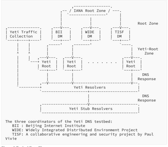
Figure 2 Testbed Data Flow
