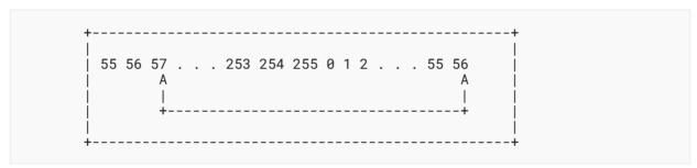
Figure 11: Sliding Samples Window
