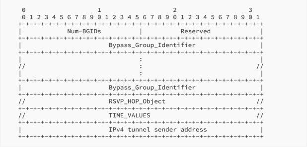
Figure 3: The IPv4 Extended ASSOCIATION ID for B-SFRR-Active
