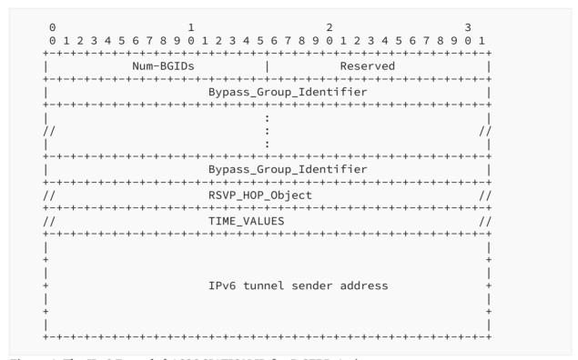
Figure 4: The IPv6 Extended ASSOCIATION ID for B-SFRR-Active
