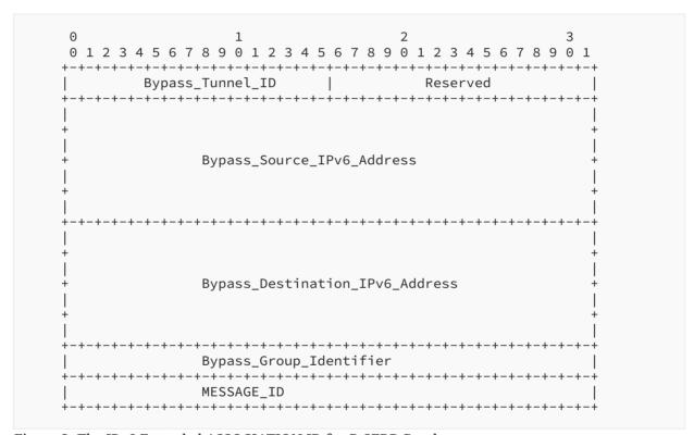
Figure 2: The IPv6 Extended ASSOCIATION ID for B-SFRR-Ready
