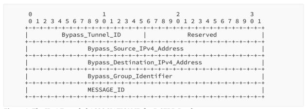
Figure 1: The IPv4 Extended ASSOCIATION ID for B-SFRR-Ready
