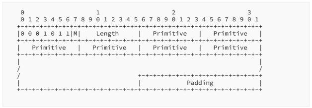
Figure 18: SUPPORTED-PRIMITIVES format
