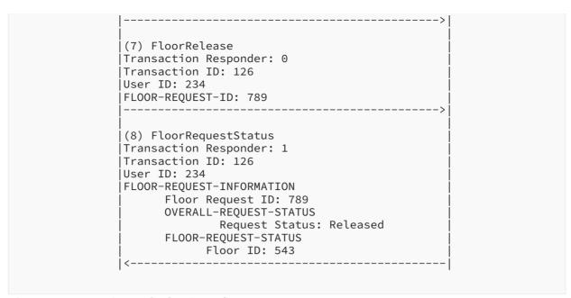
Figure 48: Requesting and releasing a floor
